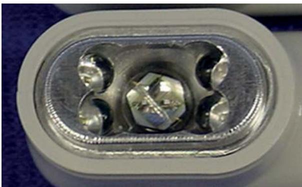
Figure 28. Image of the construction of the emitting elements in Ultradent's Ultralume 5 curing light.
