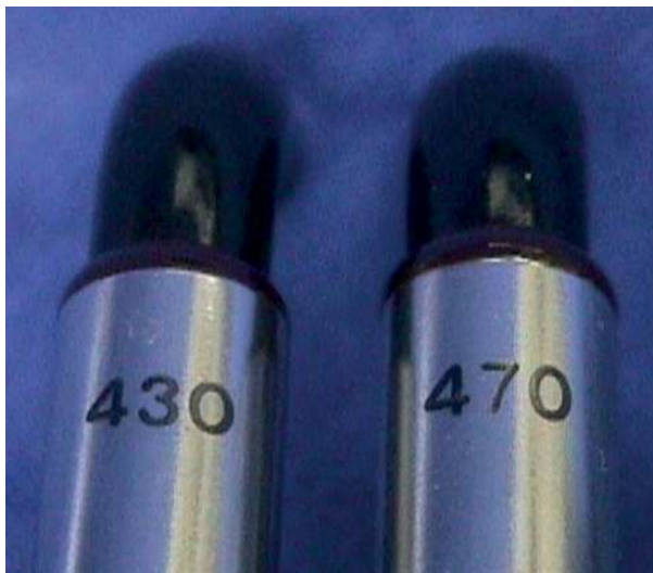
Figure 18. 430 and 460 nm tips used in early PAC lights.
