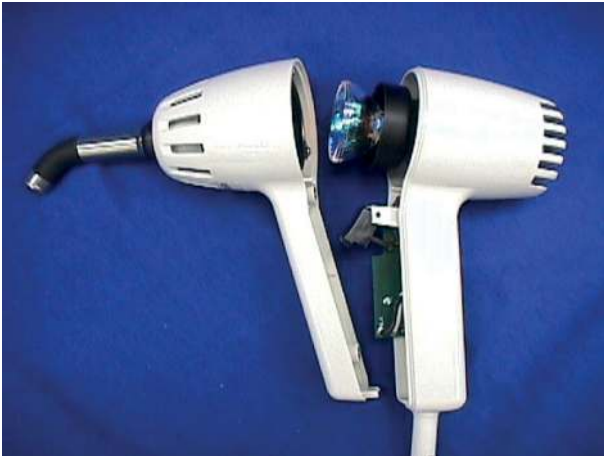
Figure 13. Internal components of a typical QTH curing light.
