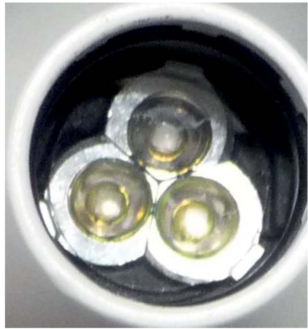
Figure 29. Image of the construction of the emitting elements in Ivoclar's Bluephase STYLE curing light.
