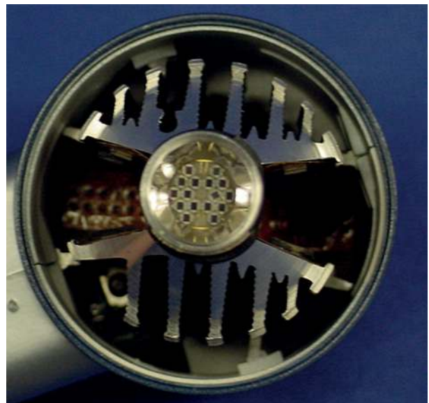
Figure 24. Small footprint area chips used in later versions of 1 st generation, blue dental light curing units.
