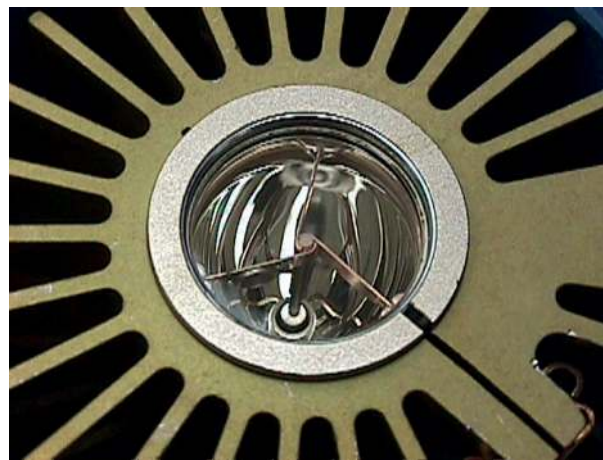
Figure 16. PAC light with associated heat sinking apparatus.
