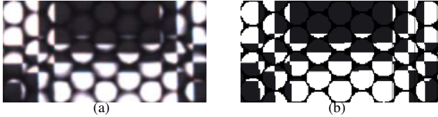
Figure 15. Zoom on a real image (a) and on a simulated image computed with the simulator using optimized projection parameters (b).
