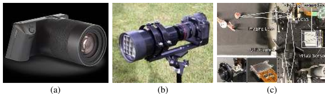
Fig. 8. Devices for multiplexed imaging. (a) Lytro Illum [4], a “plenoptic camera 1.0” that is currently commercially available. It uses a lenslet array to interlace the images of different views on a single sensor. (b) An integral camera that uses a 4 \times 5 array of lenses and prisms to capture a low angular resolution light field developed by Georgiev et al. [30]. The angular resolution can be upsampled by view interpolation techniques. (c) Marwah et al. [33] described an attenuation mask-based scheme for frequency multiplexing capture. Different samples in the light field were encoded into different frequency bands.
