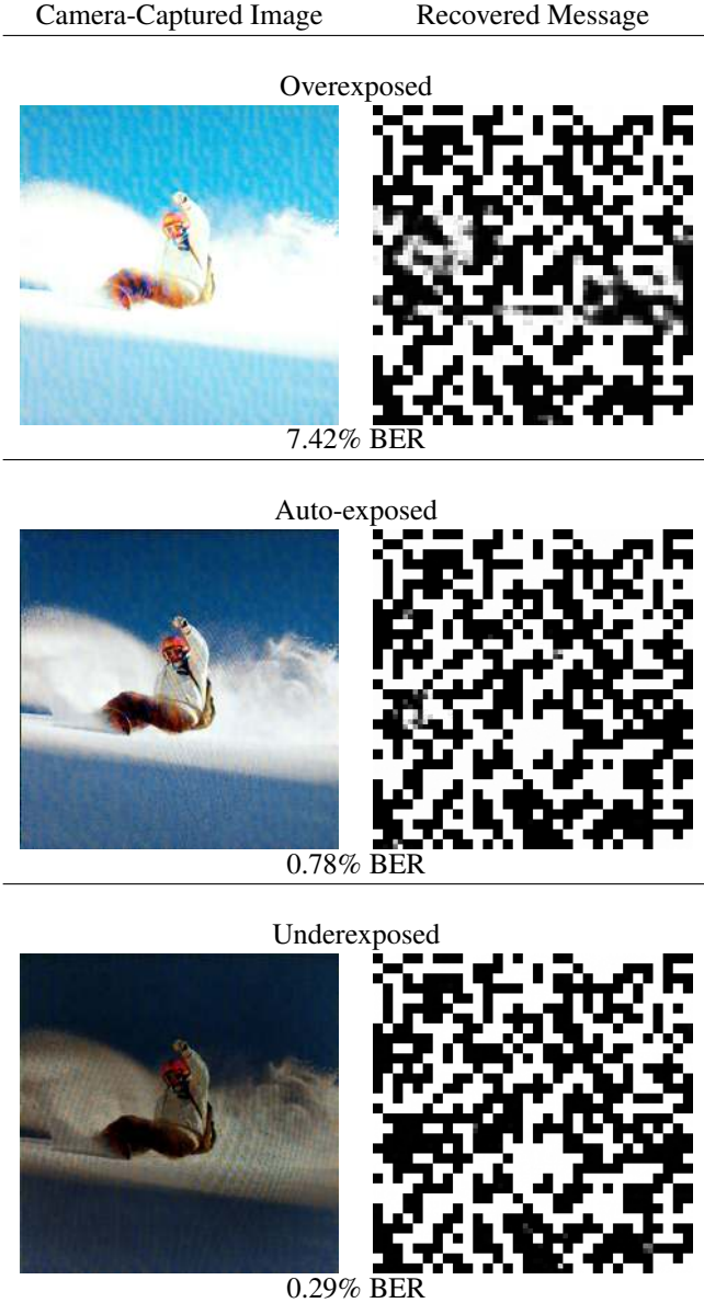
Figure 7. Our approach is robust to modifications of camera exposure, yielding low BER for multiple settings. Underexposure performs better than overexposure because the message cannot be recovered from the saturated snow pixels in the overexposed image. This experiment was performed using the Pixel 2 camera and Acer Predator XB271HU display.
