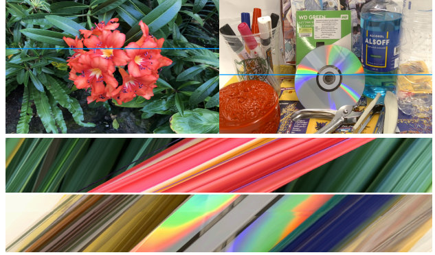
Figure 6. Epipolar-plane images (EPI). Our model represents the 4D light field, so constructing EPIs is natural. Each EPI vertically stacks images along the blue line, while the camera moves parallel to the blue line. Different depths show as lines of different slopes in the EPI, while view-dependent effects show as curves.
