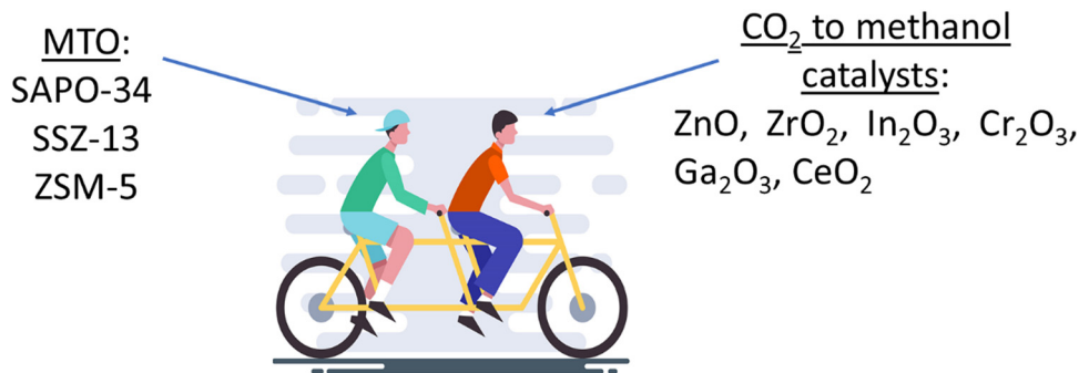
Fig. 25 Components of the tandem catalysts for LO synthesis from CO 2 : mixture of methanol synthesis and MTO catalysts.
