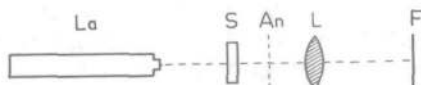
Figure 9. Schematic diagram of the laser set-up. La = laser; S = sample; An = analyser; L = lens; F = photographic plate in the focal plane of L.
