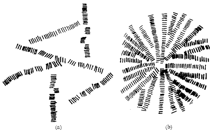
Figure 3. Schematic representations of orientation fluctuation and correlation of optical axes (indicated by lines) of anisotropic scattering elements; (a) rodlike orientation correlation, and (b) spherulitic orientation correlation.
