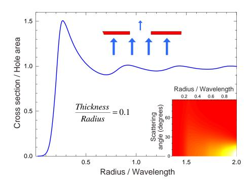
Fig. 2. Transmission cross section of a cylindrical hole in a perfect-metal slab as a function of the hole radius. The slab thickness is 0.1 times the radius. The cross section is normalized to the area of the hole, and the radius is normalized to the wavelength. The incidence of the light is perpendicular to the slab. The contour-plot inset shows the polar angle distribution of transmitted light as a function of hole radius (brighter regions stand for higher transmission intensity).
