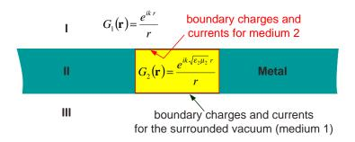
Fig. 1. Boundary element method approach to the transmission through a small hole. The problem is solved in terms of magnetic boundary charges and currents distributed around the hole boundary. See text for more details.
