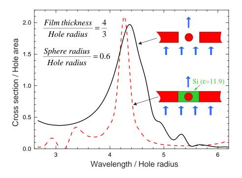
Fig. 5. Transmission cross section of a cylindrical hole drilled in a perfect-metal thin film and containing a perfect-metal sphere in its center (solid curve). The light is coming perpendicular to the film. The broken curve corresponds to the transmission of the same geometry but with the hole filled with Si (see insets).
