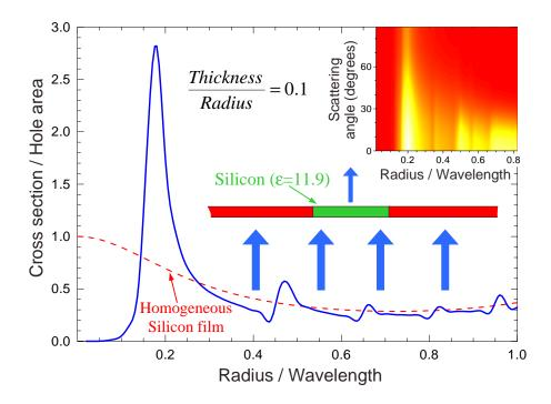
Fig. 4. Transmission cross section of a cylindrical hole drilled in a perfect-metal thin film and filled with Si (solid curve) as a function of hole radius. The broken curve represents the transmittance of a homogeneous Si film of the same thickness. The dependence of the transmitted intensity on the polar angle upon exit is shown in the inset (brighter regions stand for higher transmission intensity).
