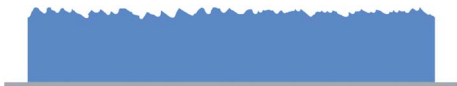
Fig. 3 A dielectric slab structure with a randomly textured front surface and a back mirror. The equivalent thickness is the same as in Fig. 2.
