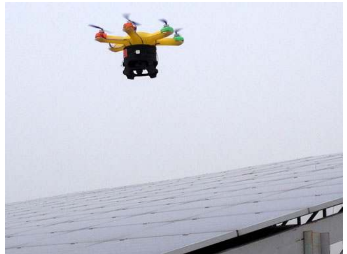
Fig. 5. Nimbus PLP6 during PV monitoring operation.
