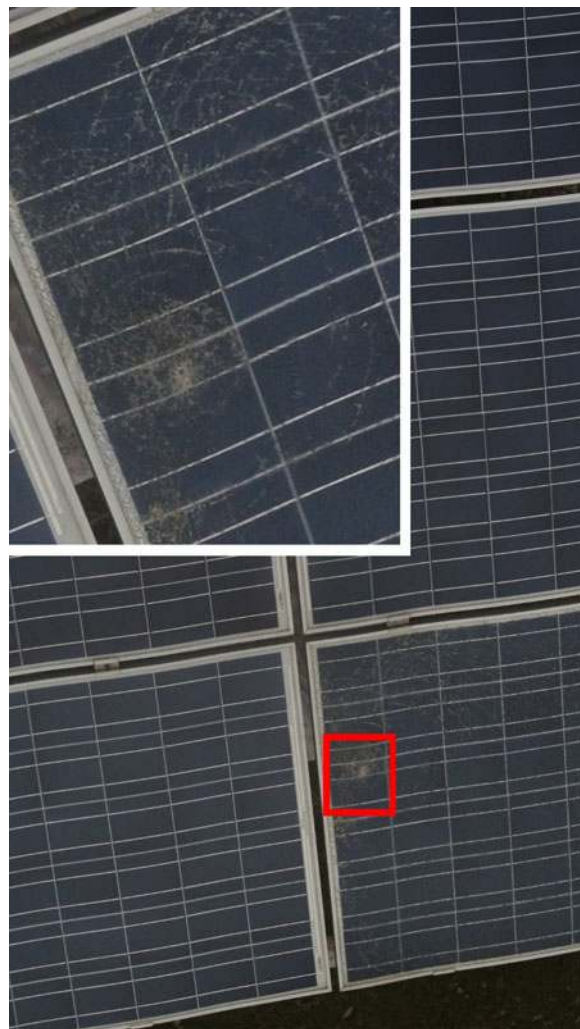
Fig. 9. Picture captured by a Nikon1-v1 camera with inlet detail of a particular shock-defect.
