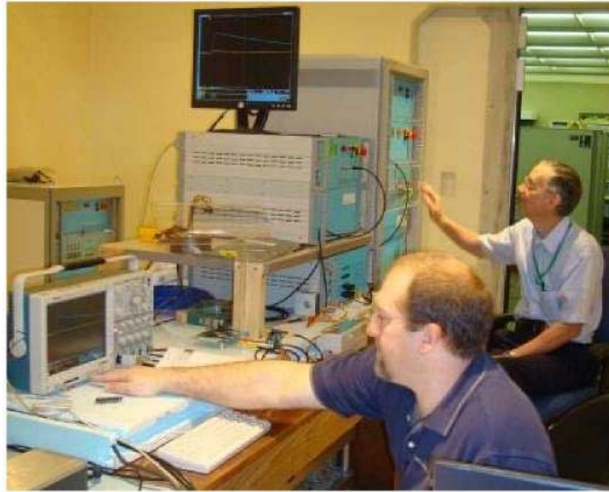
Figure 3: EMC Partner lightning-generating equipment was used for pin-injection tests.
