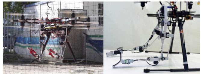
Figure 1. Dual arm aerial manipulation system consisting in two 5-DOF human size arms integrated in an octo-rotor platform.
