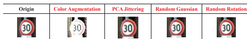
Fig. 4: From left to right: Origin picture; Color Augmentation processing; PCA Jittering processing; Gaussian Augmentation processing; Rotation Augmentation processing.
