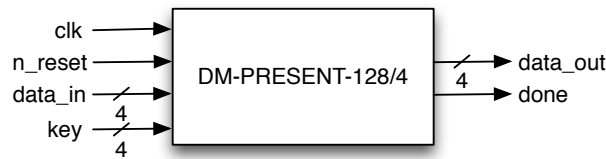
Figure 6.8: Input and output signals of the DM-PRESENT-128 top module with a datapath of 4 bits.
