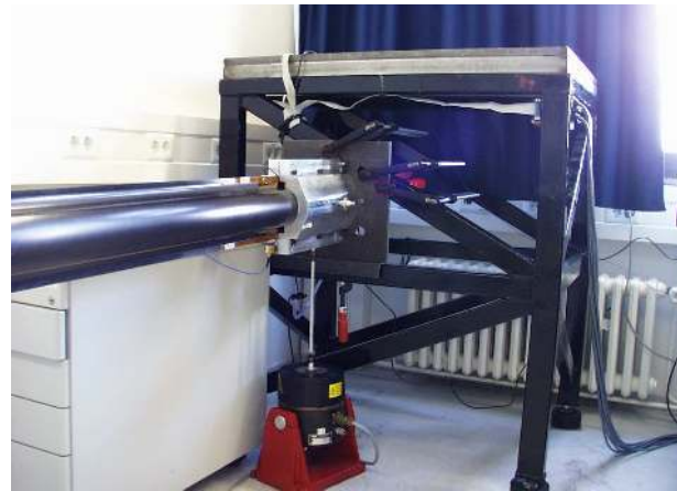
Fig. 10: Test stand with the adaptive boom supported in cantilever form (length approx. 2 m).
