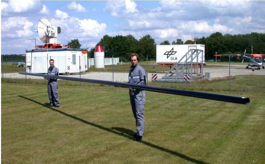
Fig. 1: Deployable CFRP boom. Length 14 m, mass 1.4 kg.
