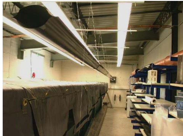
Fig. 8: Development testing on a coated boom section within the solar simulator chamber of the DLR. Structural bending test with 14 m long Solar Sail booms.
