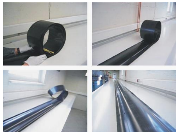
Fig. 2: The internal deformation energy of a stowed boom package enables the self-deployment of the 14 m long boom.
