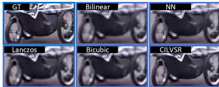
Figure 6. Visual comparison of 3\times upsampling results on image sample “Walk”, ground truth (GT), bilinear, nearest neighbor, Lanczos [58], bicubic [57], and CILVSR.
