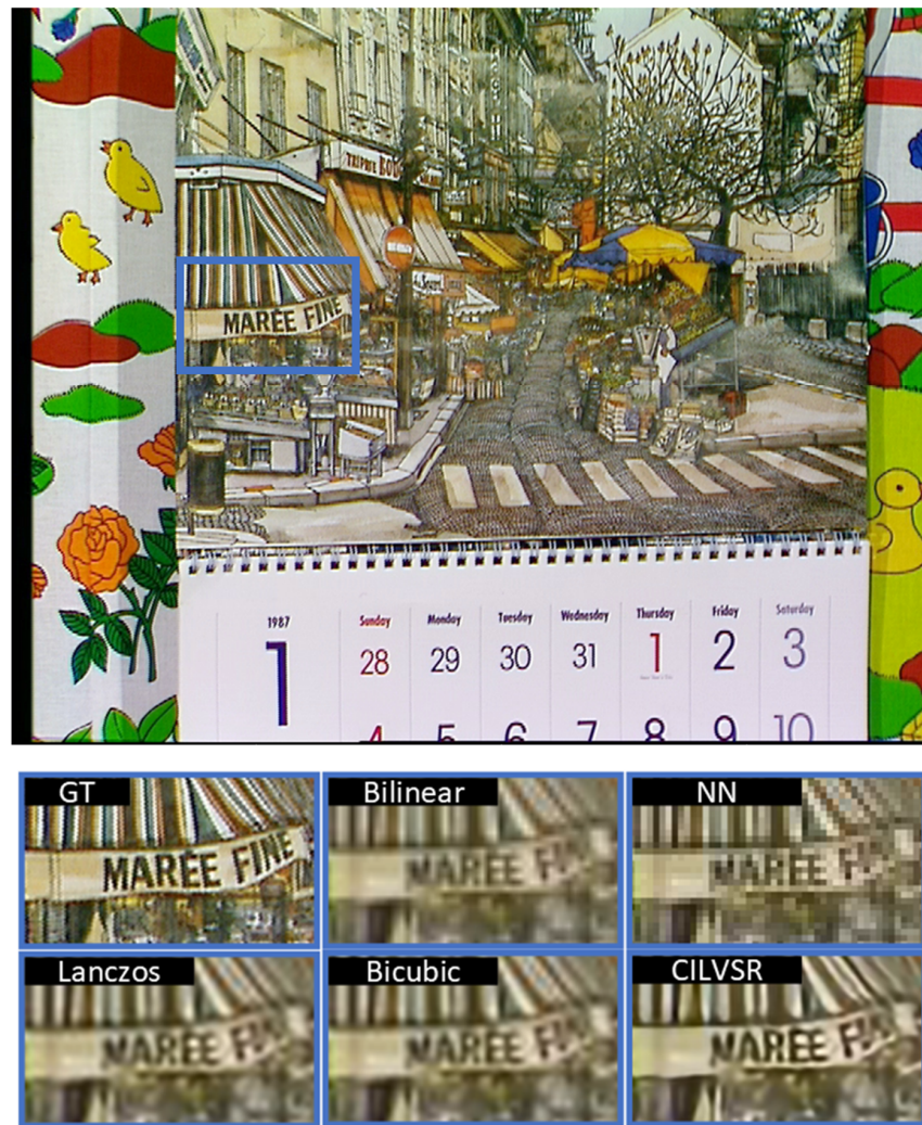
Figure 5. Visual comparison of 3× upsampling results on image sample “Calendar”, ground truth (GT), bilinear, nearest neighbor, Lanczos [58], bicubic [57], and CILVSR.
