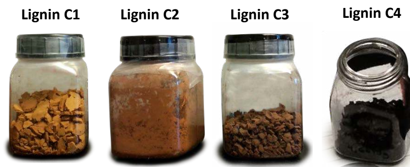
Figure 3.6. Organosolv lignin obtained from C1 to C4.
