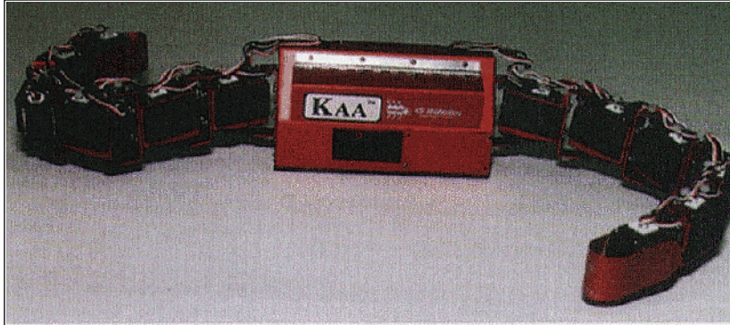
Figure 2-18: The Kaa snake is a self-contained locomoting device.
