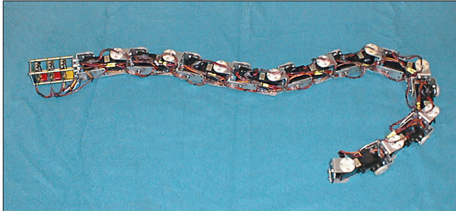
Figure 6-11: 3D snake utilizes 10 links with 20 servos
