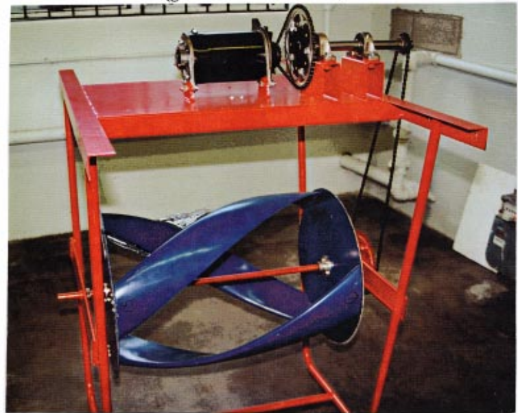
Triple-Helix Turbine (generator above water)
