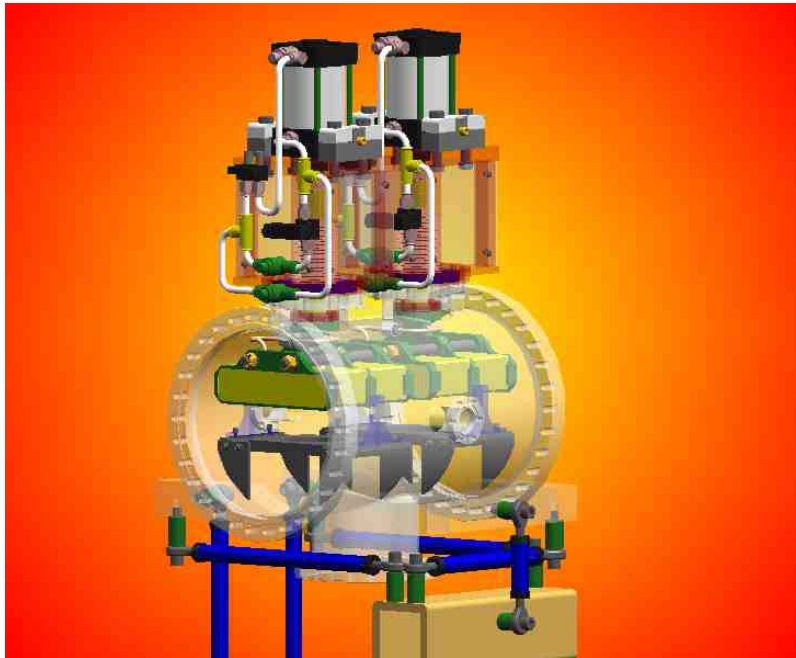
Figure 9.9 Concept of the insertable beam stop with burn-through detector.
