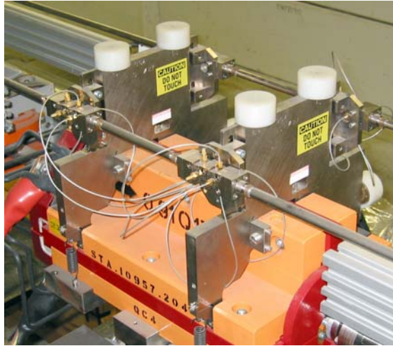
Figure 12.12 Wire Position Monitoring System
