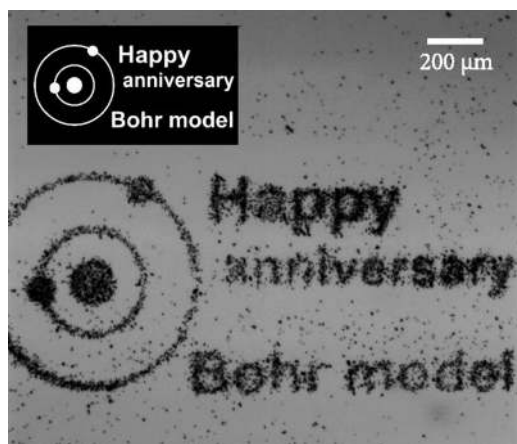
FIG. 16. 2D pattern obtained from a suspension of charged particles deposited by electrophoretic forces on a z -cut lithium niobate crystal; the inset shows the corresponding light pattern. The microscope image shows that charged particles adhere well to the previously illuminated regions without any anisotropy. Reprinted with permission from Appl. Phys. Lett. 103 , 061115 (2013). Copyright 2013 AIP Publishing LLC.
