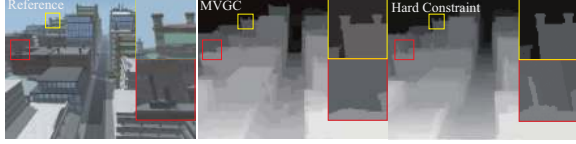
Figure 5. Encoding 3D line segments as hard constraints improves MVGC but misses important details, e.g. the chimney on the building.
