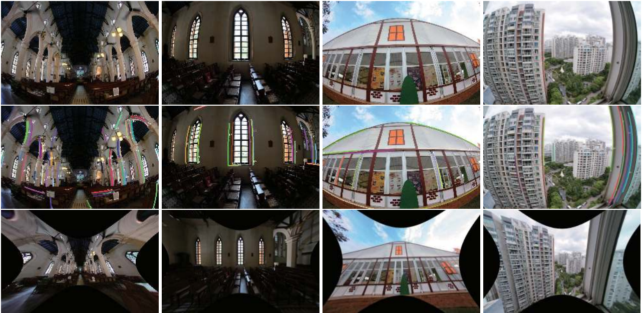
Figure 9. Rectified results of the images from the Internet: the source images downloaded from Internet in the first row, the clustered circular arcs using our proposed algorithm in the second row, and the rectified results in the last row.
