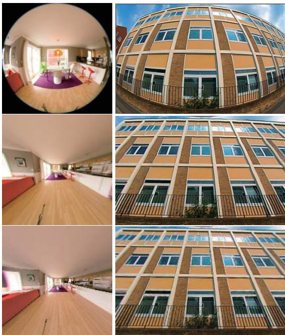
Figure 8. Rectified results of our algorithm and the commercial software DxO. From top to bottom are the source images, the manually rectified results with the commercial software DxO, and our automatically rectified results.
