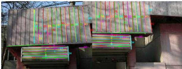
Figure 6. Results of line matching on a pair of images with occlusion. This figure is better viewed in color. Extracted Lines : 159,95. Total matches: 45, Correct matches: 45.
