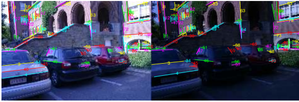
Figure 5. Results of line matching on a pair of images with brightness changes. This figure is better viewed in color. Extracted Lines : 211,131. Total matches: 97, Correct matches: 97.
