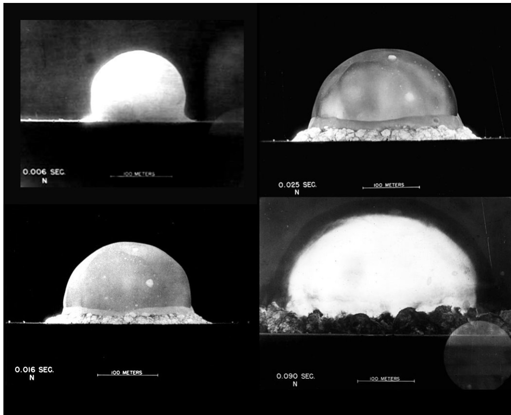
Figure 10: Time-lapse photographs with distance scales (100m) of the first atomic bomb explosion in the New Mexico desert - 5.29 A.M. on 16th July, 1945. Times from instant of detonation are indicated in bottom left corner of each photograph (Top first - left column: 0.006s, 0.016s; right column: 0.025s, 0.09s).
