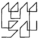
Figure 16. The Front Half of a Three-dimensional Hilbert Curve on a Cube 4 \times 4
