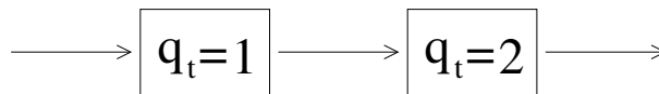
Figure 7.6: Example of a switching topology which can be used to approximate non-linear dynamics.
