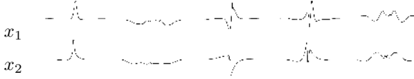
Fig. 2. Five principal basis functions for the inverted pendulum along the x_1, x_2 dimensions.
