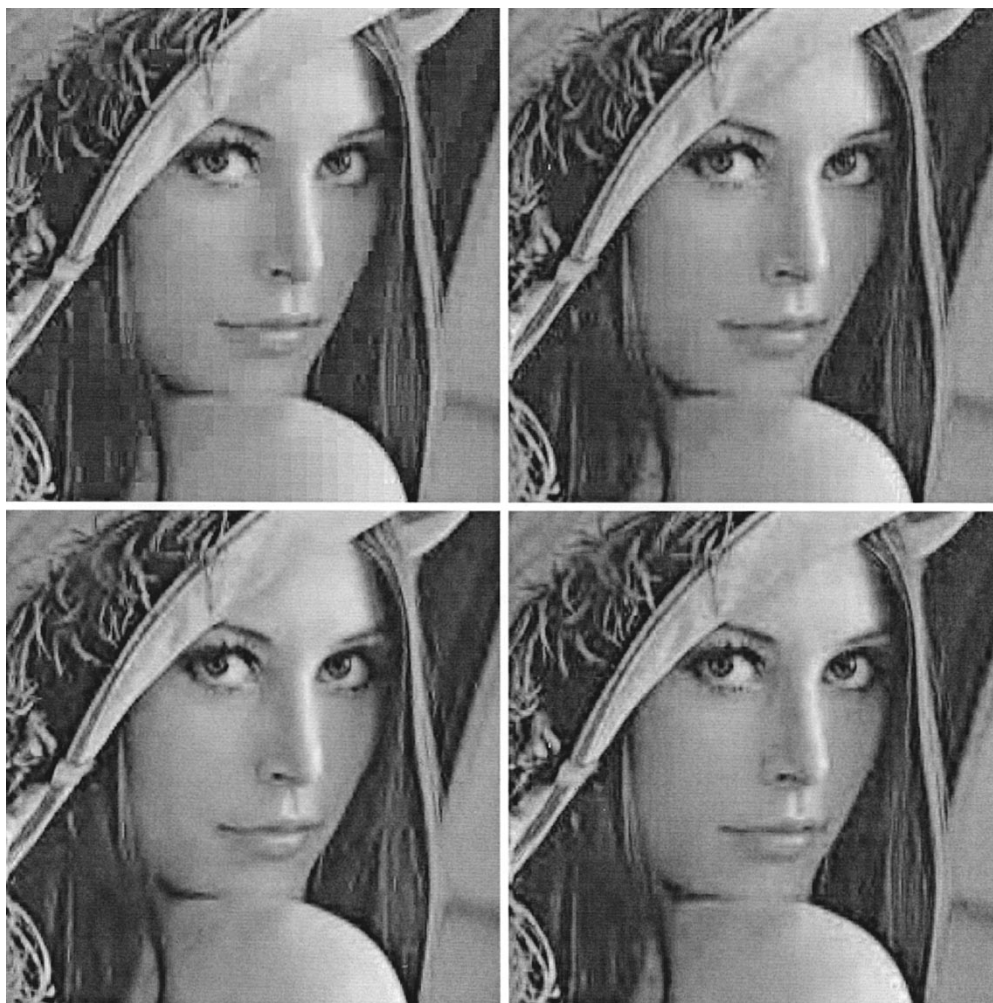
Fig. 13. Enlarged 256 \times 256 portions of reconstructed Lena images at 1:32 compression ratio. Top left: 8 \times 8 DCT. Top right: 8 \times 16 type-II fast LOT. Bottom left: 9/7-tap biorthogonal wavelet. Bottom right: 4 \times 24 \times 8 fast VLLOT.
