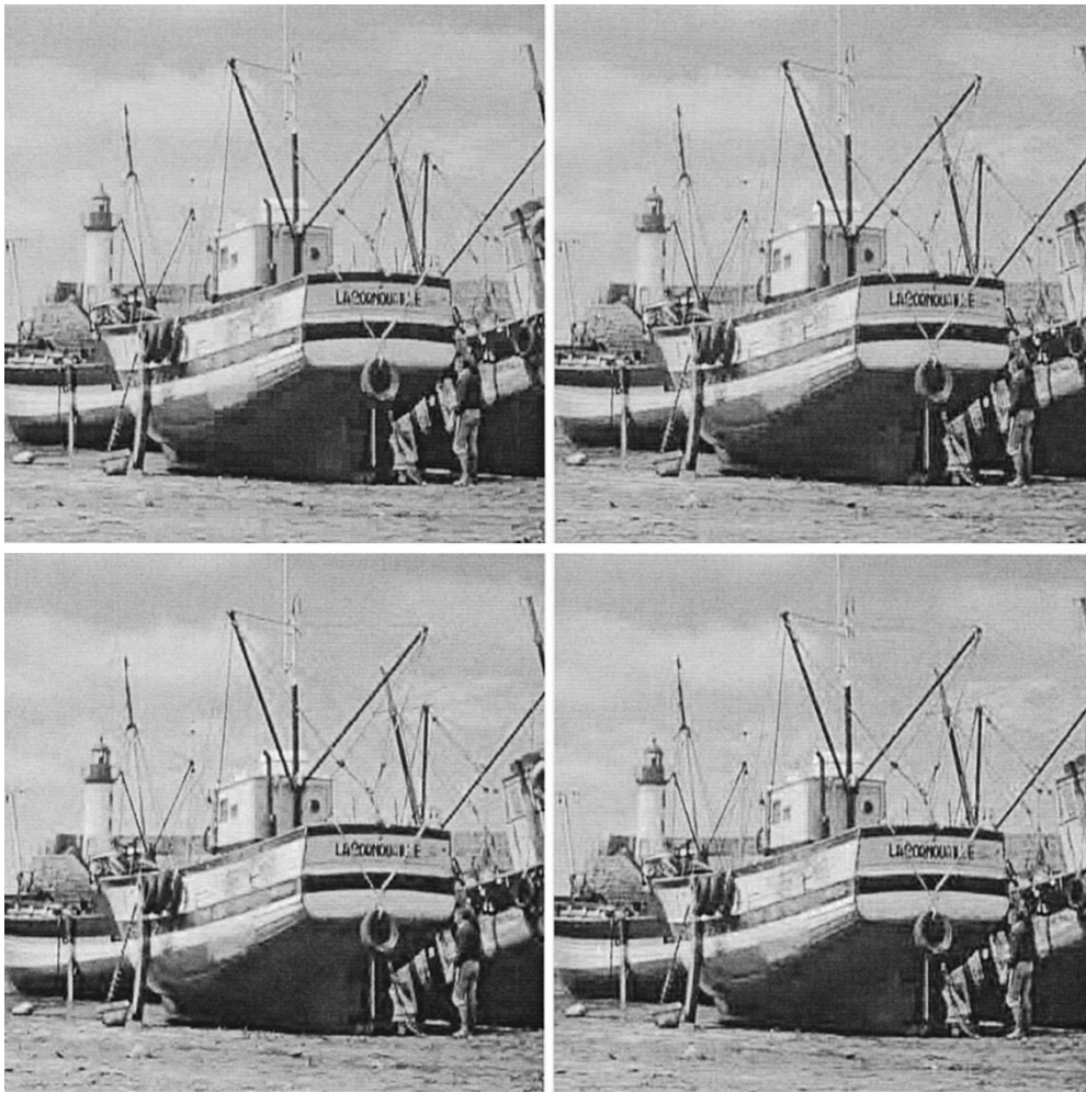
Fig. 11. Reconstructed boat images at 1:32 compression ratio. Top left: 8 \times 8 DCT, 30.43 dB. Top right: 8 \times 16 type-II fast LOT, 30.93 dB. Bottom left: 9/7-tap biorthogonal wavelet, 30.97 dB. Bottom right: 4 \times 24 4 \times 8 fast VLLOT, 30.89 dB.
