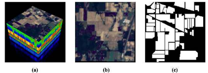
FIGURE 10: The sample of hyperspectral image (Indian Pine Site 3 AVIRIS hyperspectral dataset). (a) overview image, (b) cross section, (c) ground truth.
