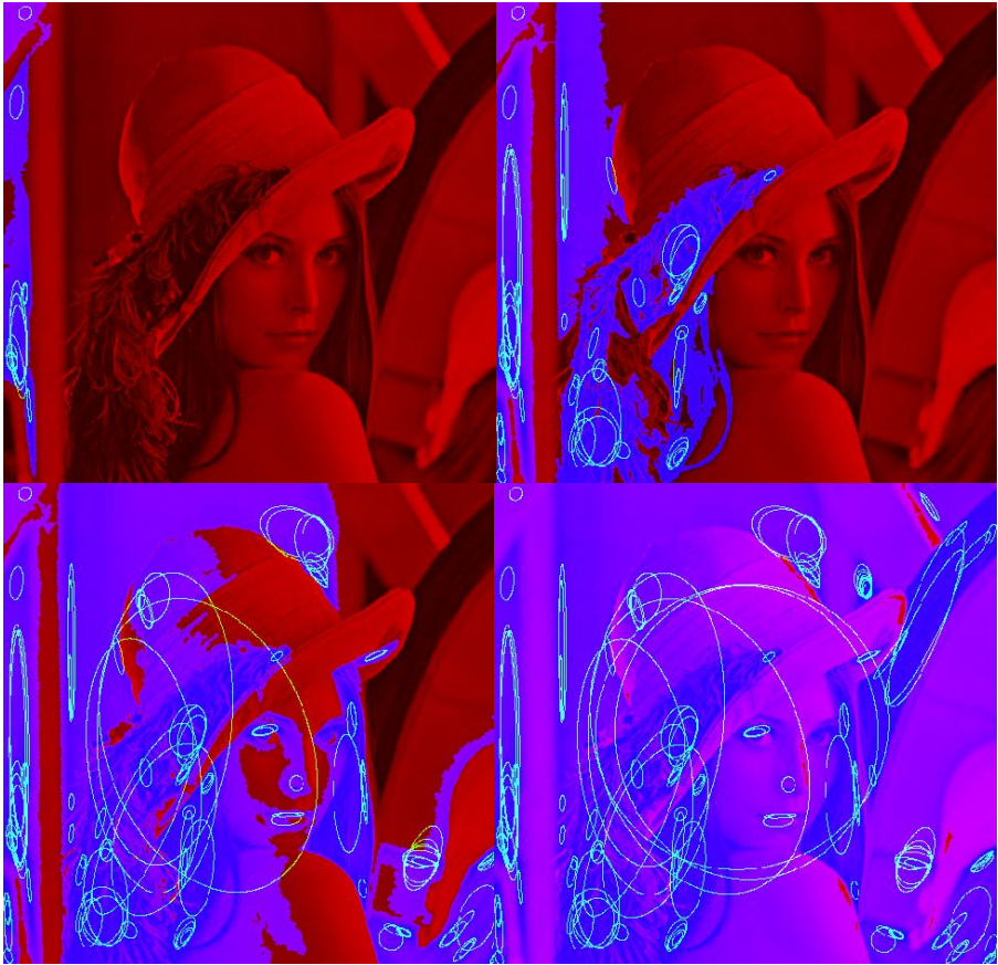
Fig. 2. Typical progress stages for the algorithm on the first pass. The top left pixel is used as the source pixel. The flooding occurs, with preference for dark regions, MSER are detected in the process, and eventually the whole image is flooded. The process will then be repeated with preference for bright regions.
