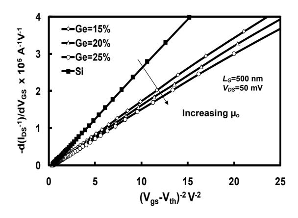
Fig. 2(a).  $\partial (I_{DS}^{-1})/\partial V_{GS}$  plotted as a function of  $(V_{GS}-V_{TH})^{-2}$  for Si control and strained Si nMOSFETs. The low field mobility is inversely proportional to the slope of the line and  $\theta_2$  can be extracted from the x-axis intercepts.
