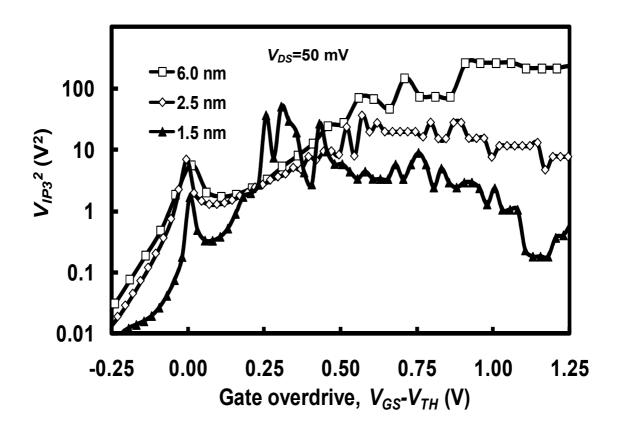
Fig. 10.  $V_{IP3}^2$  as functions of  $V_{GS}$ - $V_{TH}$  for 1.4 nm, 2.5 nm and 6 nm gate oxide MOSFETs.  $V_{IP3}^2$  increases with the oxide thickness because  $\theta_2$  reduces as oxide thickness increases.
