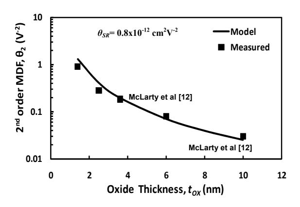
Fig. 9. The calculated and measured  $\theta_2$  values shown as functions of the oxide thickness.  $\theta_2$  increases as the oxide thickness is decreased and there is good matching between the calculated and measured data.
