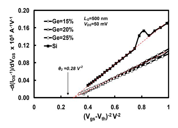
Fig. 2(b). An enlarged version of Fig. 2(a) showing the intercepts of the straight lines with the x axis. The  $2^{nd}$  order MDFs extracted for all the MOSFETs is approximately  $0.29~V^{-2}$ .
