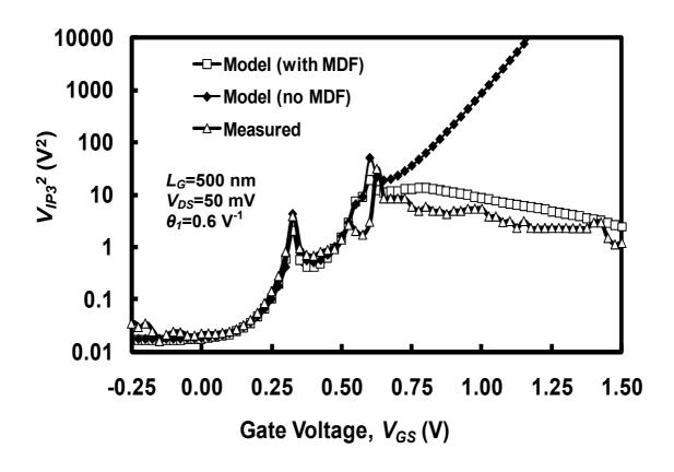
Fig. 7. A comparison of measured  $V_{IP3}^2$  characteristics and calculated  $V_{IP3}^2$  characteristics with  $\theta_2$ =0.28 V<sup>-2</sup> and  $\theta_2$ =0 V<sup>-2</sup>. There is a match between the calculated  $V_{IP3}^2$  and measured  $V_{IP3}^2$  only when  $\theta_2$  is tuned to the measured value.
