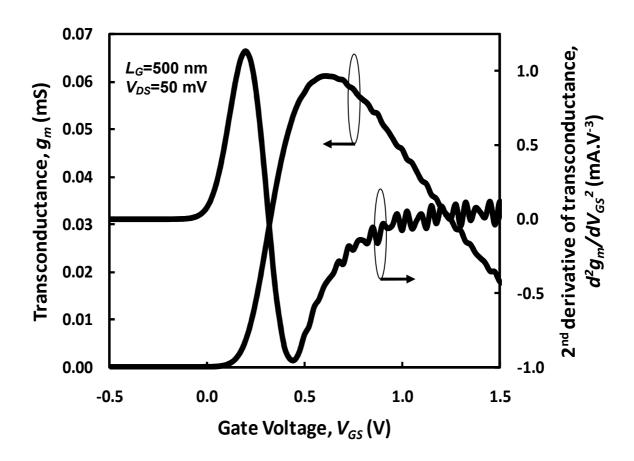
Fig. 5. Measured  $g_m$  and  $\delta^2 g_m/\delta V_{GS}^2$  as functions of  $V_{GS}$ - $V_{TH}$  for the Si control MOSFET.
