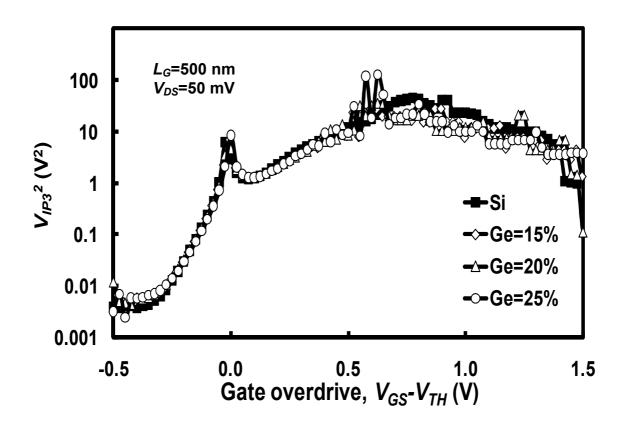
Fig. 4.  $V_{IP3}^2$  as a function of the gate voltage overdrive for strained Si and Si control nMOSFETs. There is no impact of strain on the  $V_{IP3}^2$ .
