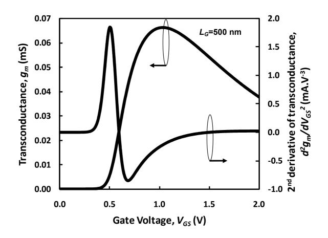
Fig. 6. Calculated  $g_m$  and  $\delta^2 g_m / \delta V_{GS}^2$  as functions of  $V_{GS} - V_{TH}$ . The semi-empirical MOSFET model is calibrated with measured parameters. A  $\theta_2$  of 0.3 V<sup>-2</sup> is required to match the shape of the calculated characteristics with the measured one.
