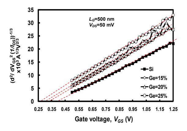
Fig. 3. The extraction of the threshold voltage from the x axis intercepts. The  $V_{TH}$  extracted reduces as the strain content increases.  $V_{TH}$  extracted agrees with values extracted using linear transconductance.
