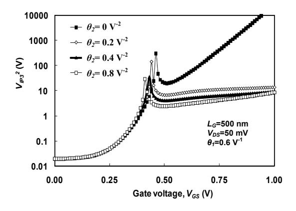
Fig. 8. The calculated  $V_{IP3}^2$  characteristics shown as functions of  $\theta_2$ .  $V_{IP3}^2$  reduces significantly as  $\theta_2$  increases. The linearity can be overestimated without taking  $\theta_2$  into account.
