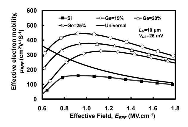
Fig. 1. The effective mobility as a function of the vertical effective field for the Si control and strained Si nMOSFETs on  $Si_{1-x}Ge_x$  SRBs for x=0.15, 0.20 and 0.25. The effective mobility is proportional to strain.
