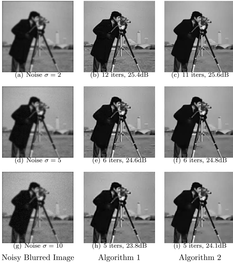
FIG. 4.3. Deblurring results of Algorithms 1 and 2 for 256 \times 256 cameraman image convolved by a 15 \times 15 Gaussian kernel of \sigma_b = 2 generated by the MATLAB command fspecial('Gaussian',15,2) and contaminated by a Gaussian white noise of variance \sigma^2 .
