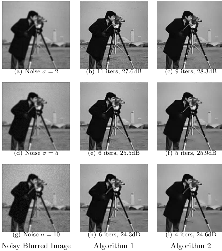
FIG. 4.1. Deblurring results of Algorithms 1 and 2 for 256 \times 256 cameraman image convolved by a 7 \times 7 disk kernel generated by the MATLAB command fspecial('disk',3) and contaminated by a Gaussian white noise of variance \sigma^2 .
