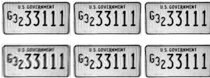
FIG. 4.8. Comparison of intermediate iteration steps of the iteration in Algorithm 1 with iteration (4.4) for the image deblurring in Fig 4.7 with \sigma = 2 . The top row shows the 10th, 20th, and 50th iteration steps of the iteration in Algorithm 1. The bottom row shows the 10th, 100th, and 1000th iteration steps of (4.4).
