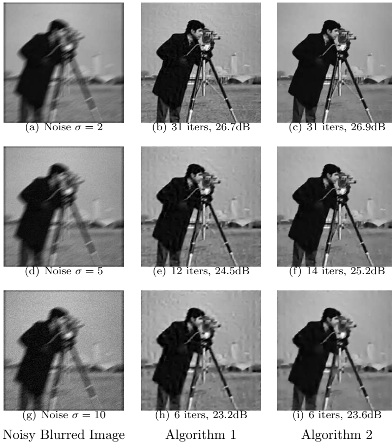
FIG. 4.2. Deblurring results of Algorithms 1 and 2 for 256 \times 256 cameraman image convolved by a 9 \times 15 motion kernel generated by the MATLAB command fspecial('motion',15,30) and contaminated by a Gaussian white noise of variance \sigma^2 .
