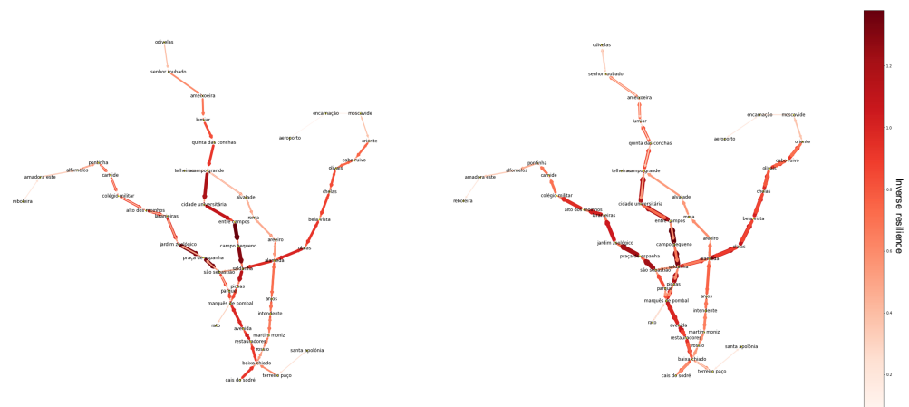
Figure 12. METRO lean resilience using supply and demand on the 15 October 2019 at 9 A.M. on the left and 5 P.M. on the right.
