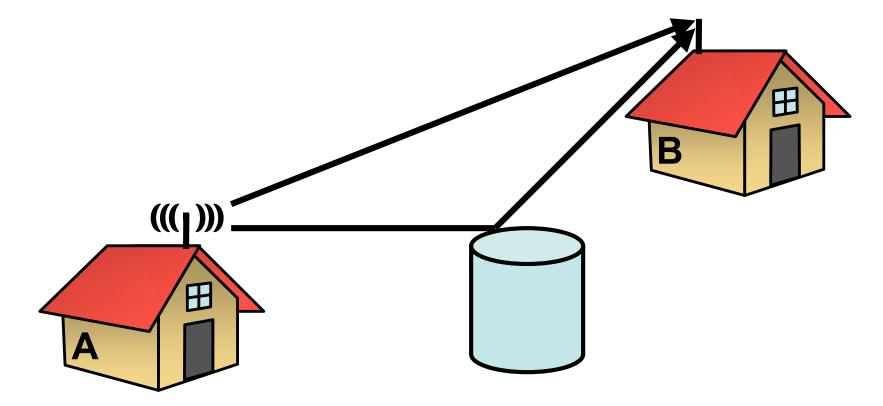
Reflection is a delayed and attenuated copy of the signal
