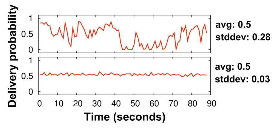
The top graph is consistent with bursty interference. The bottom graph is not.
