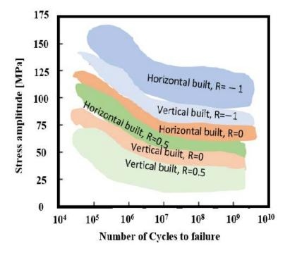
**Figure 19.** A plot of stress amplitude vs. number of cycles to failure for AlSi10Mg specimens fabricated with different orientations and tested under different stress ratios [109].
