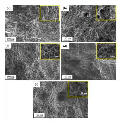
**Figure 17.** Fracture surfaces of specimens built in the horizontal direction: (**a**) as-built, (**b**) annealed, and after (**c**) HP + T6, (**d**) HIP + T6, and (**e**) T6 treatment. The magnified images are provided in the yellow boxes located at the top right corner. Reprinted with permission from Ref. [64]. Copyright 2020 Springer Nature.
