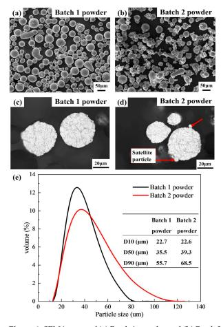
**Figure 4.** SEM images of (**a**) Batch 1 powder and (**b**) Batch 2 powder. Polished cross-sections showing (**c**) spherical particles in Batch 1 powder and (**d**) satellite particles in Batch 2 powder. (**e**) The particle size distribution of Batch 1 and Batch 2 powders. Reprinted with permission from Ref. [47]. Copyright 2021 Elsevier.
