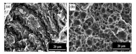
**Figure 16.** High magnification SEM images of the fractured surfaces of the (**a**) as-built and (**b**) heat-treated specimens. Reprinted with permission from Ref. [32]. Copyright 2016 Elsevier.
