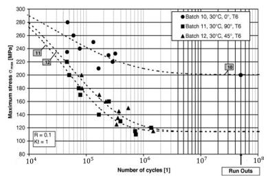
**Figure 14.** Fatigue resistance and Weibull distribution (50% probability of failure) of specimens built at 30 °C platform temperature. Reprinted with permission from Ref. [15]. Copyright 2012 Elsevier.
