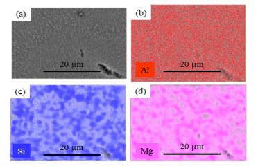
**Figure 8.** (a) SEM image of a representative AlSi10Mg specimen with EDX maps of (b) Al, (c) Si, and (d) Mg. Reprinted with permission from Ref. [53]. Copyright 2017 Elsevier.
