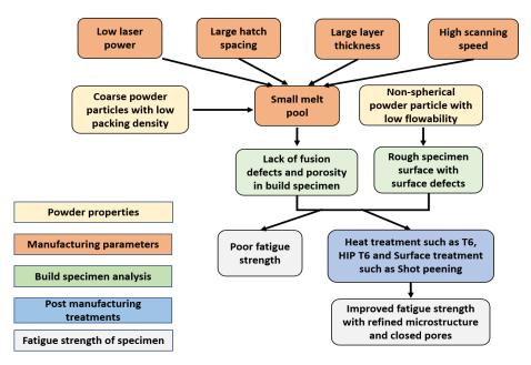
**Figure 18.** A schematic illustrating the impact of powder properties and printing parameters on the fatigue properties.
