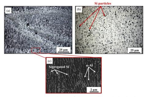
**Figure 15.** Representative optical images of AlSi10Mg in the (**a**) as-built and (**b**) heat-treated conditions. (**c**) High-magnification SEM image of the as-built microstructure revealing Si segregation on the boundaries of  $\alpha$ -Al. Reprinted with permission from Ref. [32]. Copyright 2016 Elsevier.
