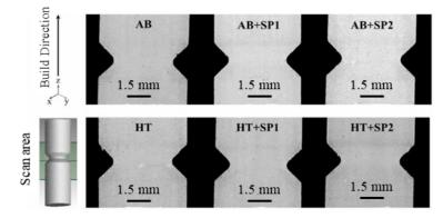
**Figure 20.** CT images of the sub-surface porosities around the notches. Reprinted with permission from Ref. [100]. Copyright 2022 Elsevier.
