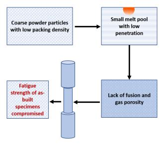
Figure 11. Schematic depicting the impact of porosity on fatigue strength.
