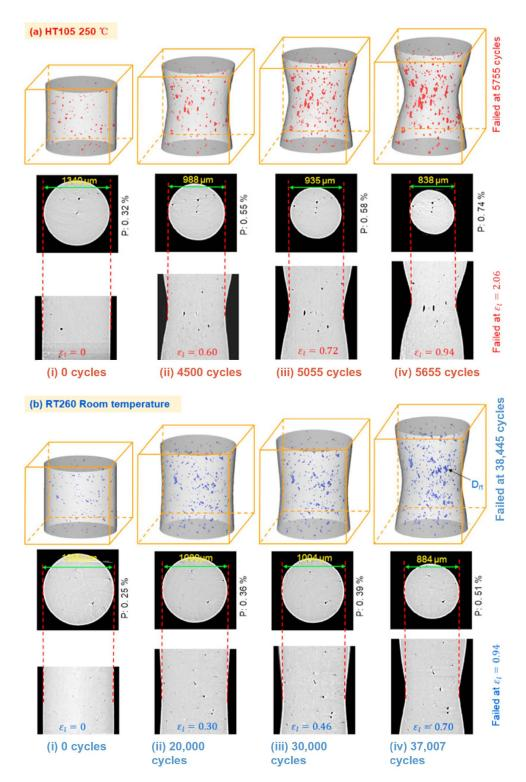
**Figure 21.** Time-lapse images of (**a**) the specimen (HT105) tested at 250 °C and peak load of 105 MPa and (**b**) the specimen (RT260) tested at room temperature test and peak load of 260 MPa as a function of numbers of cycles showing the 3D rendering of the voids (**top**), a virtual mid-plane slice (**middle**), and a diametrical slice (**bottom**) in each case. Reprinted with permission from Ref. [113]. Copyright 2020 Elsevier.
