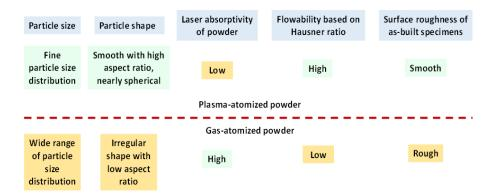
Figure 3. Overview of powder properties obtained by gas and plasma atomization.
