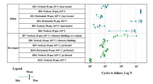
**Figure 12.** Impact of contour and build direction on the fatigue resistance of AlSi10Mg. Fatigue testing was conducted at a stress amplitude of 120 MPa and with a stress ratio of -1. Reprinted/adapted with permission from Ref. [82]. Copyright 2018 Elsevier.
