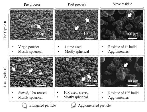
**Figure 5.** Representative SEM images of the AlSi10Mg powders: pre-process (**left**), post-process and sieved (**middle**), and sieved residue (**right**) for the virgin powder (**upper**) and 10th use cycle (**lower**). Reprinted with permission from Ref. [51]. Copyright 2021 Laboratory for Freeform Fabrication and University of Texas at Austin.
