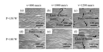
**Figure 7.** OM images showing the melt pool morphology of AlSi10Mg specimens processed at different laser power and scanning speeds. Here, 'P' represents the laser power and 'v' represents the scanning speed. Reprinted/adapted with permission from Ref. [53]. Copyright 2017 Elsevier.
