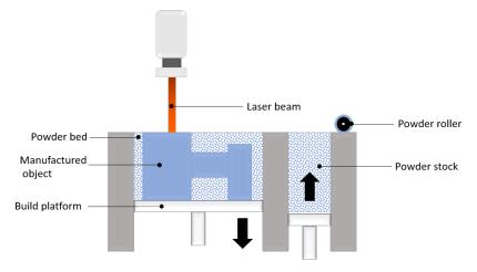
Figure 1. Schematic of an L-PBF process.
