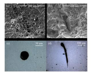
**Figure 9.** (**a**,**c**) Representative gas porosities. (**b**,**d**) Lack of fusion porosities. Reprinted with permission from Ref. [71]. Copyright 2020 Elsevier.
