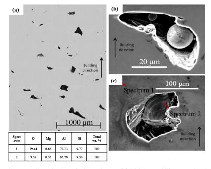
increased. Such a rise in oxygen content was confirmed by the SEM/EDX analysis of specimens built using reused AlSi10Mg powder, as shown in Figure 6.
