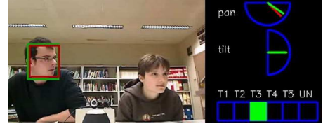
Figure 3: Tracking, head-pose estimation, and VFOA estimation for a meeting participant.
