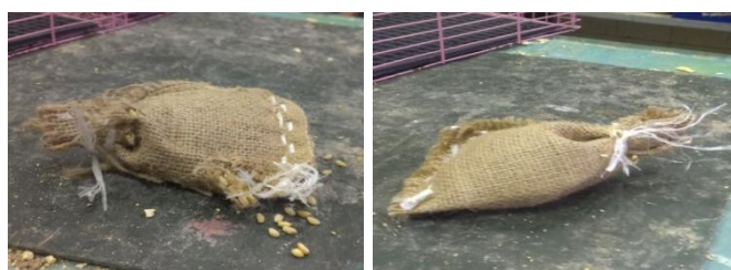
Fig. 9: Photography image of untreated and treated burlap (4x4 inch) filled with wheat. a) Zero time of exposure, b) untreated after penetration (24 h of exposure) and c) treated after penetration (24 h of exposure).
