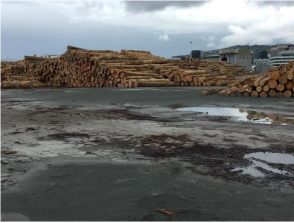
Figure 11: Sandy liquefaction ejecta in the log stacking area (hydraulic fill reclamation) in the northeast corner of CentrePort (Sample S13). (S41.274972° E174.788347°, taken on 17 NOV16).
