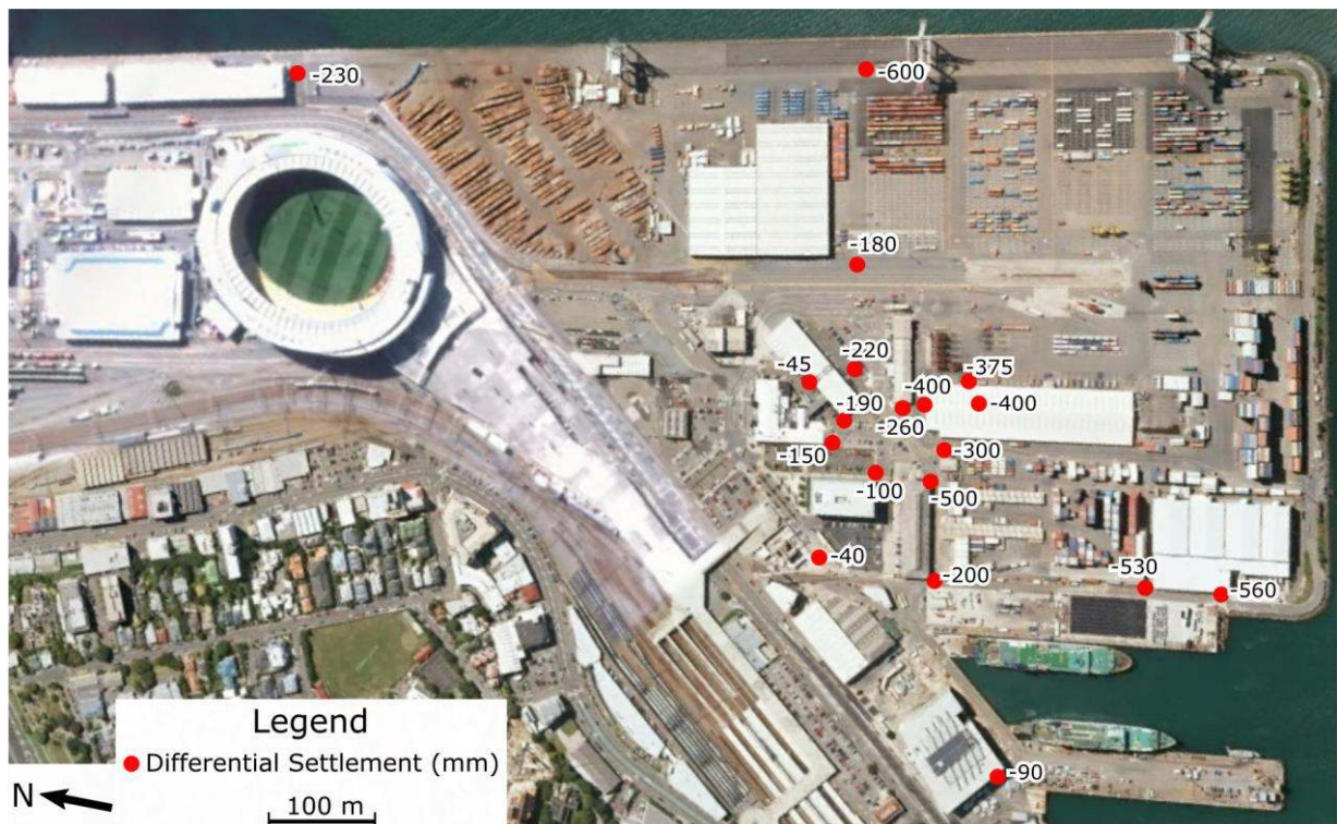
Figure 14: Location and magnitude of differential settlement measurements obtained during inspections. All values are in mm, and represent settlement of the ground surface relative to a pile supported structure (Base image from Google Earth™).
