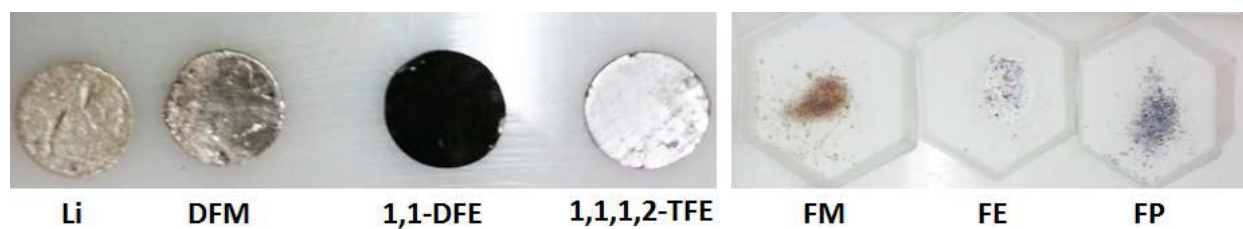
Figure S5. Optical images of lithium metal after submersion in liquefied gas solvents. Reaction products as a result of submerging lithium metal in six different liquefied gas solvents, with bare lithium metal (left most image) for comparison. All samples were submerged in solvent till all chemical reaction activity was seen to cease, times which are tabulated in Table S2 .
