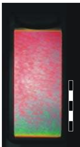
Figure 7.9 – Early stage of the rotation of a nematic phase in a horizontal magnetic field, used in Chapter 5 to determine \Delta n_{sat} . Sample thickness d = 2.00 mm, B = 1.4 T, the scale bar denotes 1 cm. The temporal periodicity observed in this sample hints at the same type of transient pattern as observed in the much thinner samples in this study. However, the initial alignment of this sample was not homeotropic, hence, we do not draw quantitative conclusions from this observation.
