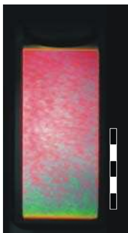
Figure 7.9 – Early stage of the rotation of a nematic phase in a horizontal magnetic field, used in Chapter 5 to determine \Delta n_{sat} . Sample thickness d = 2.00 mm, B = 1.4 T, the scale bar denotes 1 cm. The temporal periodicity observed in this sample hints at the same type of transient pattern as observed in the much thinner samples in this study. However, the initial alignment of this sample was not homeotropic, hence, we do not draw quantitative conclusions from this observation. (See colour version at page 138.)
