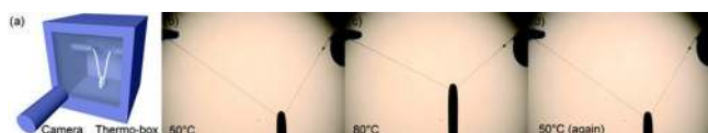
Figure 43. Schematic setup (a) and results (b) of a heating experiment performed on a single SmA LCE filament, glued between two static substrates inside a heatable metal box. A small, U-shaped weight was clipped to the sample. The temperature in the box was cycled while observing the sample with a camera. Between 50 (b) and 80 °C (c) the weight was lifted up while the substrates remained stationary. Upon cooling back to 50 °C (d) the sample went back to its original height, proving the reversibility of the actuation. Reproduced from [311] with permission of The Royal Society of Chemistry
