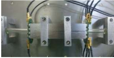
a) The installed ECT sensor with metal cover.
