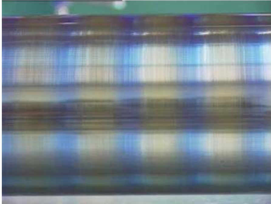
Figure 6.10: Photograph of the barber pole flow pattern. The fluids are equal volumes of water and kerosene.
