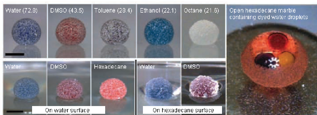
Figure 7 Encapsulation of low surface tension liquids and use as miniature reactors. Reprinted with permission from ref. 19. Copyright 2010 Wiley-VCH Verlag GmbH & Co. KGaA.
