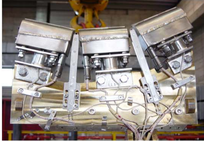
Figure 7. Photograph of the FTU liquid lithium limiter . The multilayer molybdenum mesh retention system is at top, in three sections, with the lithium reservoirs and heating system into each section, below the mesh surface.
