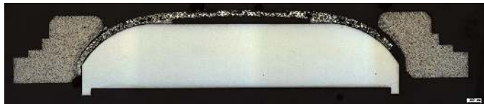
(b) Cut through sample, after exposure in PSI-2
