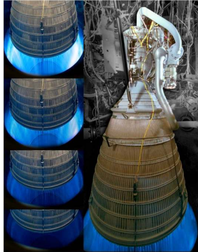
Common Extensible Cryogenic Engine (CECE) at Varying Thrust (2005)
