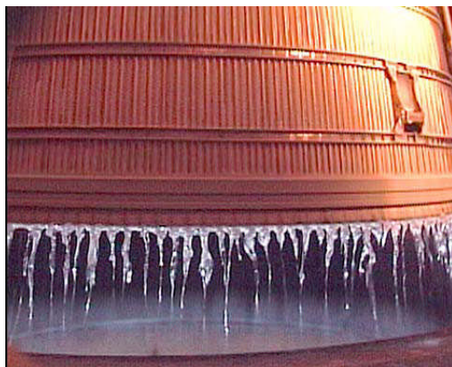
Figure 7. CECE at 30% Power Levels Showing Ice Formation
