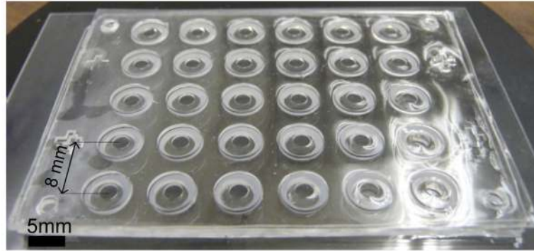
Figure 10. Optical image of the structure of one microlens array without filling the lens liquids. The array consists of 5×6 microlenses. Reprinted from [69] with permission from Institute of Physics .
